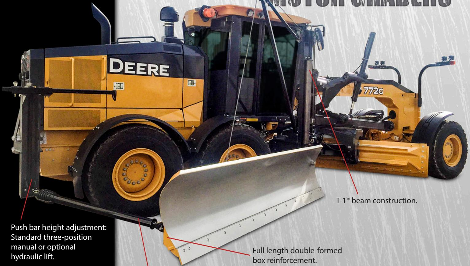
Push bar height adjustment: Standard three-position manual or optional hydraulic lift.
