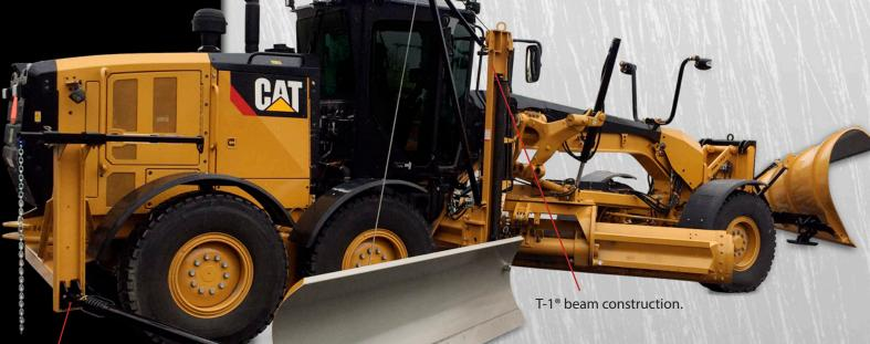
Push bar height adjustment: Standard three-position manual or optional hydraulic lift.
