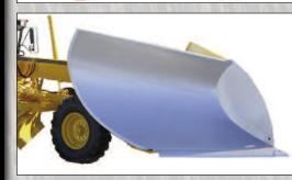
Shoe adjustment, including nose shoe, is made easily without the use of tools.
